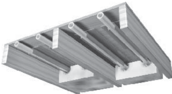
Below subfloor installation
